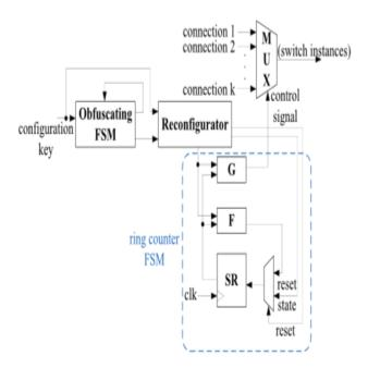
Fig 2 Complete reconfigurable switch design
